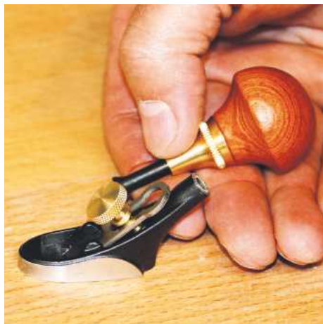
▲ The handle can be removed to use as a finger plane
